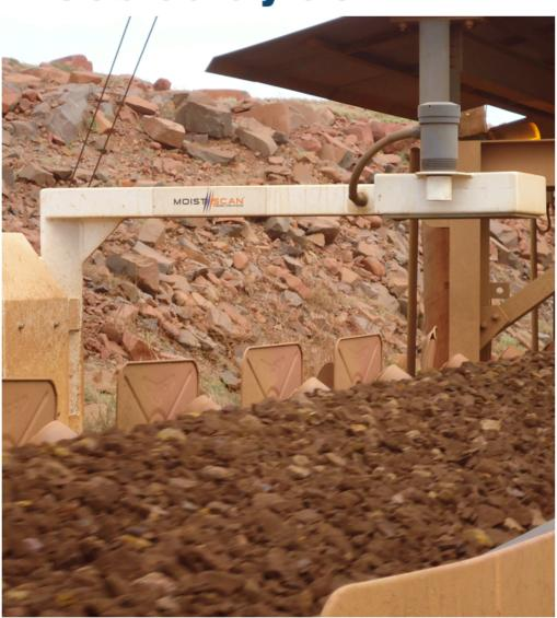
industry understanding the benefits of onbelt microwave monitors being used to provide operators with moisture analysis of their ore every minute. For example, if plants have regular, minute by minute analysis of the moisture content of the incoming ROM, then down-stream processes may be adjusted to achieve greater efficiencies and in fact, increase
